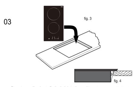
Do not use adhesive to fix the hob into the worktop. Once the seal is fitted position the hob into the cutout in the worktop. Apply gentle downwards pressure onto the hob to push it into the worktop ensuring a good seal around the outer edge (fig. 4)
