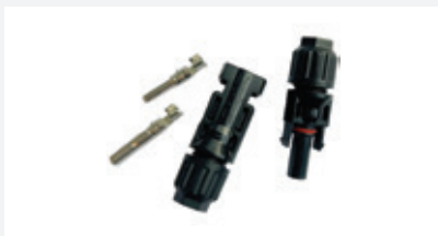
MC4 DC Solar Cable Connectors For cables 2.5mm² to 6.0mm², 30A max current, max voltage 1000V. IP68.
